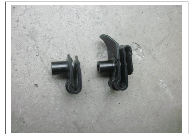
Figure 14: Cut down lower bumper clips for use on rear of inner guard
