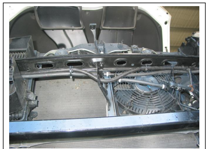
Figure 6: Wiring and headlight washer loome attachment under grille support.
