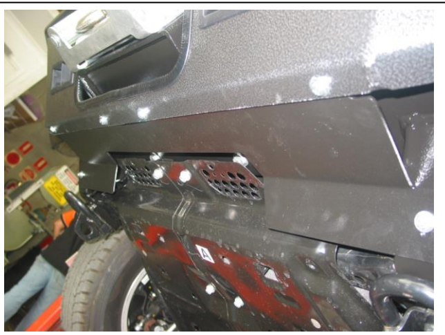
Figure 19: Centre under body guard fitted.
